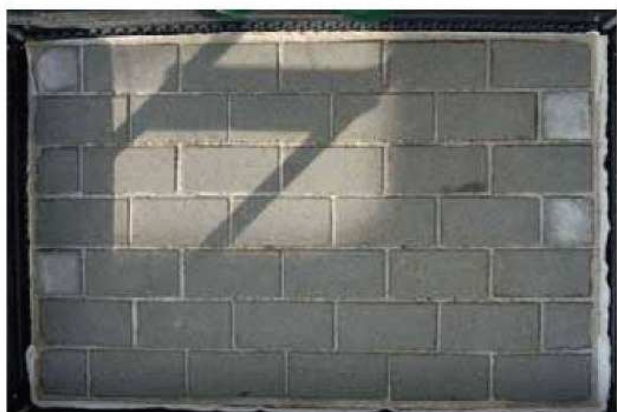
Figure 6: In the dry trial, the sections with Dorfner Fugensand+ are almost free of vegetation (Photo taken on 21.04.2010,
