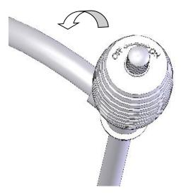
off, turn it anticlockwise. This way you empty the siphon pump.
