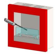
Insert the lighter tube into the hole and set fire to the bioethanol;
