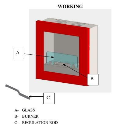
The fireplace exclusively works with bioethanol. The burning is regulated by the rod (C). The bioethanol feeding take places as follows:
