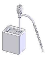
Turn clockwise (ON position) the knob at the > Dip the rigid pipe inside the bioethanol tank and the flexible pipe inside the fireplace tank.
