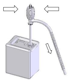
Exercise various pressures on the siphon bulb >> Finish filling the fireplace tank, turn the knob  $\triangleright$ until the bioethanol starts coming out.
