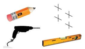
Mark the 4 holes positions with the aid support bracked; and proceed with drilling and inserting appropriate dowels to the type of wall;
