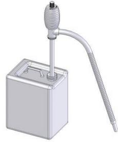
Dip the rigid pipe inside the bioethanol
