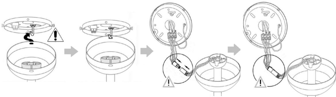
6. Fixed the top cap and adjust the down rod to right position.
