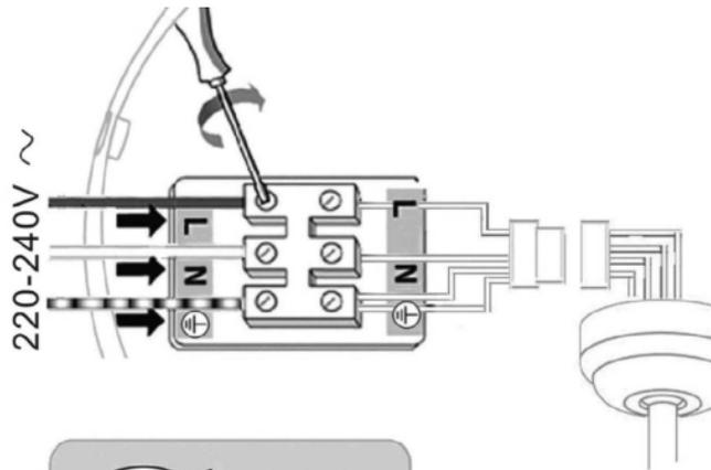
3. Disassembly the down rod and insert the wires with terminal through inside of down rod.
