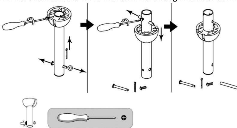
4. Assembly the down rod with motor housing and the top cap.
